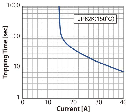
Measurement environment: No airflow, 25 ± 1°C
